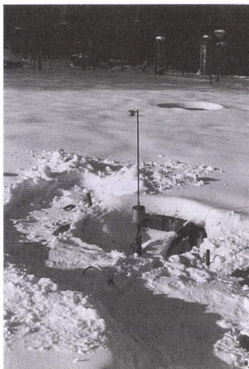
Fig. 10. The radioactive collector of the equipment by means of which the atmospheric electric potential gradient is measured
