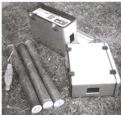
Fig. 8. On-line audiomagnetotellurics instrument (Ádám et al. 1988)
