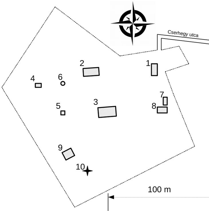
**Fig. 2.** Schematic of the buildings, measurements operate at the THY. 1 Clock house; 2 Absolute house (absolute pillars [1 and 2] and total field measurement); 3 Variation house (pillars are in the eastern and in the western room); 4 Pavilion (two pillars); 5 New measurement hut; 6 Temperature hut; 7 Test building; 8 Laboratory; 9 Green house; 10 VLF antenna.
