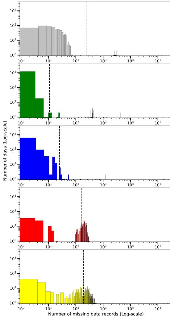
**Fig. 6.** Distributions of the number of missing data records per stations. The grey, green, blue, red and yellow colors from top to bottom indicate station COBS, SOPGO, SOPPAL, BREBA and PTNA, respectively. The dashed vertical lines represent the average value of missing records due to the failure of data transmission and recording (column 7, Table IV).
