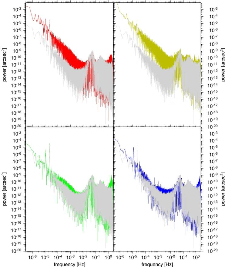
**Fig. 3.** Comparison of PSDs of N–S ground tilt time series observed at the monitoring stations of the Mur–Mürz fault line. The PSD of data recorded at COBS is the reference (grey), the other curves show PSDs of SOPGO (green), Soppal (blue), BREBA (red) and PTNA (yellow) stations.
