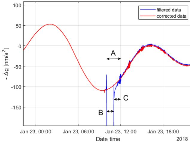
**Fig. 12.** Gap due to sticking of the index beam to one side of the measuring range caused by a large magnitude earthquake and its correction in the gravimeter measurements. Interval A: Filled/interpolated gap, Interval B: Data gap due to temporal index beam sticking. Interval C: Relaxation period after the index beam freely moves again.
