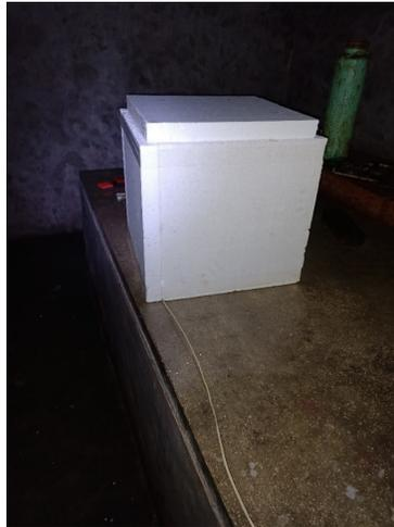
**Fig. 2.** A typical insulation hut of the tiltmeters applied at most sites.
