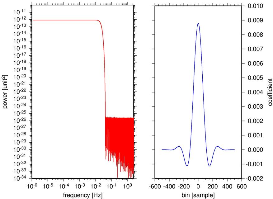
**Fig. 11.** The frequency (left panel) and time (right panel) representations of the low-pass GGP filter (`gls1md`) used to eliminate high frequency noise from the tilt observations recorded at 5 Hz sampling rate.
