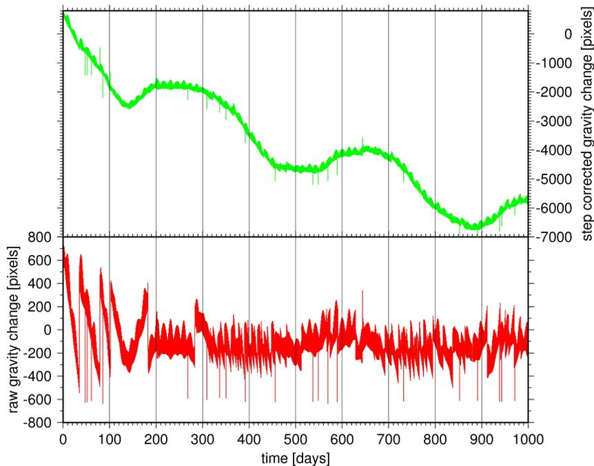
**Fig. 9.** A thousand days long time series of gravity variations recorded at COBS between 2017–2020 before (bottom panel) and after (top panel) step corrections. The waving shapes on the diagrams are the indications of the harmonic tidal signal.
