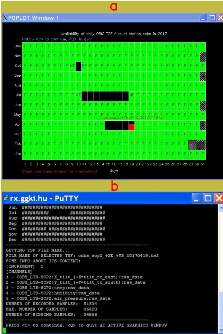
**Fig. 8.** (a) A calendar like presentation of the availability of the daily TSF files recorded by the SOP2 sensor at COBS in 2017. F: full, NF: not full. The height of the red column on the 19<sup>th</sup> of April is proportional to the number of available data. (b) Some details about the selected TSF file (cobs\_sop2\_+XE\_+YS\_20170419.tsf) and the data stored in it.
